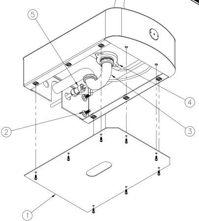
Remove the drinking fountain bottom access panel (1). Set the access panel aside in a safe place where it will not be damaged and place the screws in a secure location where they will not be lost.
